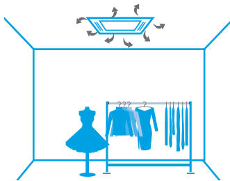
Air distribution with a dusty filter
